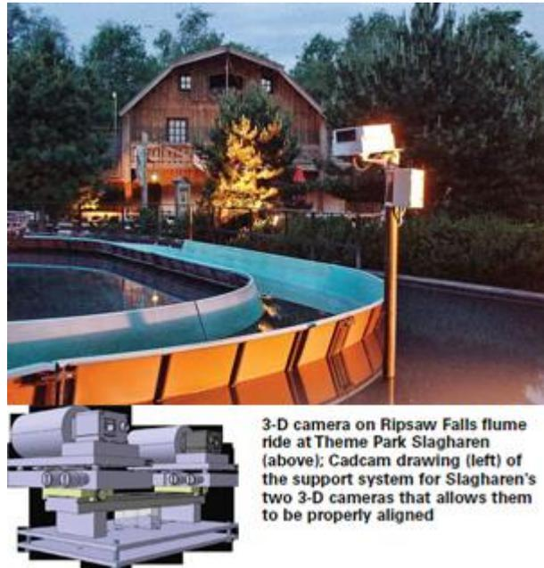
3-D camera on Ripsaw Falls flume ride at Theme Park Slagharen (above); Cadcam drawing (left) of the support system for Slagharen's two 3-D cameras that allows them to be properly aligned
